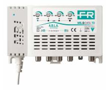
1-input (III+DAB+IV+V) multiband TV indoor amplifier with 35dB gain and up to 120dBµV output level on UHF band, separate bands amplification with independent level adjustment (20dB) for each band and low noise figure. T2 technology with UHF cut band for LTE 4G @790MHz and 5G @694MHz.
